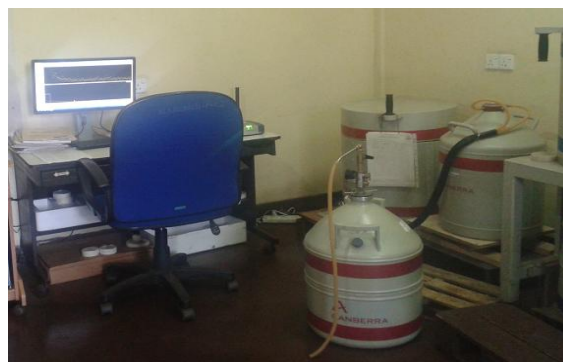
Fig.8.1: Ultra background High Pure Germanium Detector system in the Low Level Counting Laboratory
