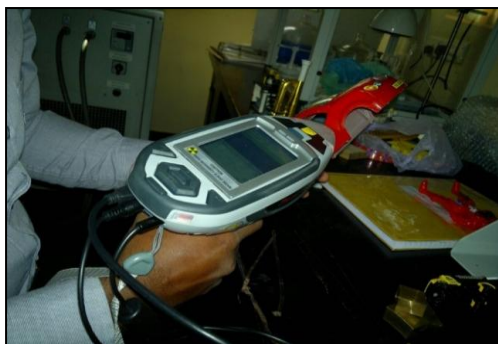
Fig.8.6: Sample analysis using portable XRF instrument
