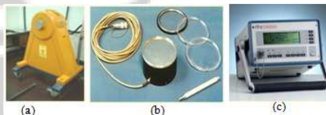
Figure 1: (a) OB85 Gamma Irradiator (b) 600 cc thin window ionization chamber (c) Electrometer (PTW, UNIDOS)
